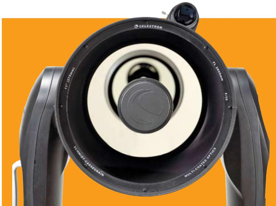
**THE CPC 1100 GPS** is an 11-inch f/10 Schmidt-Cassegrain telescope. Its focal length is 2,800 millimeters, which means the supplied 40mm eyepiece yields 70x. With this scope, you'll see stars as faint as magnitude 14.7; its theoretical resolving power is 0.42". All optics receive Celestron's Starbright coating, which increases light throughput.
