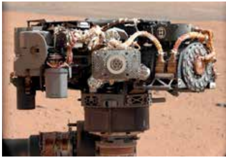
Curiosity's Mast Camera snapped this portrait of the rover's Alpha Particle X-Ray Spectrometer (APXS). Scientists directed the camera to take the image to determine whether APXS had been covered in dust during the rover's landing.
