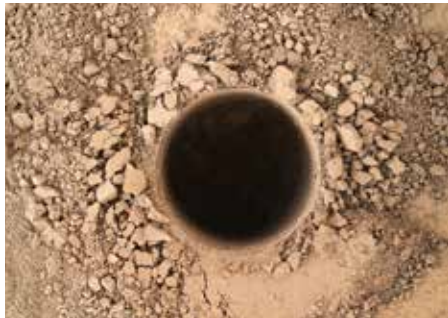
Curiosity continues to explore the layered rocks on Mount Sharp's lower slopes. In September 2014, the rover drilled its first hole on the mountain to collect samples for onboard analysis. The hole measures 0.63 inch (1.6 centimeters) across and 2.6 inches (6.7cm) deep. NASA/JPL-CALTECH/MSSS
