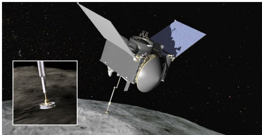
OSIRIS-REx will reach out its sample collector like a vacuum cleaner extension (inset) to gather samples from asteroid Bennu's surface, possibly retrieving up to a few pounds. NASA GODDARD SPACE FLIGHT CENTER
