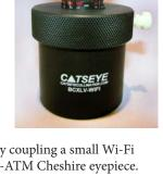
nate that back-and-forth process by coupling a small Wi-Fi camera with their BLACKCAT XL-ATM Cheshire eyepiece. The camera sends an image you can view on the included app, allowing you to tweak the primary's collimation while seeing the Cheshire's ring/center spot reflections directly on your iOS or Android smartphone's screen. Note: The app is not compatible with Android version 12.
