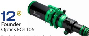
Founder Optics' 106mm f/6 triplet refractor is unique both inside and out. The multicoated objective consists of three fully gapped elements. Two are made of extra-low dispersion (ED) glasses (S-FPL 53 and S-FPL 51), while the third is made of lanthanum. The glossy black tube and green anodized rings, carrying handle, and 2.7" focuser really stand out. Also included are a field flattener for photography and an aluminum carrying case.
