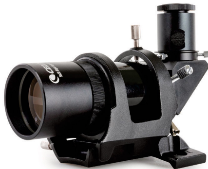
Celestron's Right Angle Correct Image Finderscope features a 2-inch (50mm) front lens and a magnification of 9x. Its right-angle design offers a more comfortable viewing position than a straight-through finder scope. CELESTRON
