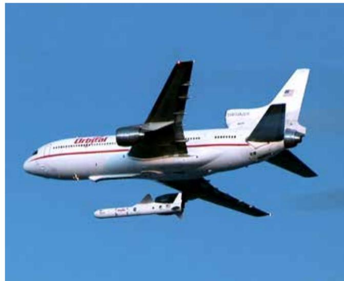
NuSTAR was launched from a Pegasus rocket strapped to the belly of Orbital Science's Stargazer aircraft in 2012. ORBITAL SCIENCES CORPORATION
