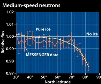
MESSENGER's neutron spectrometer surveys the entire planet looking for neutrons. If no ice existed on Mercury, the number of neutrons would remain constant with latitude. If the radar-bright deposits were pure ice, the plot would follow the yellow curve. The MESSENGER data closely match the pure-ice scenario. ASTRONOMY: RICK JOHNSON, AFTER NASA/JHUAPL/CIW
