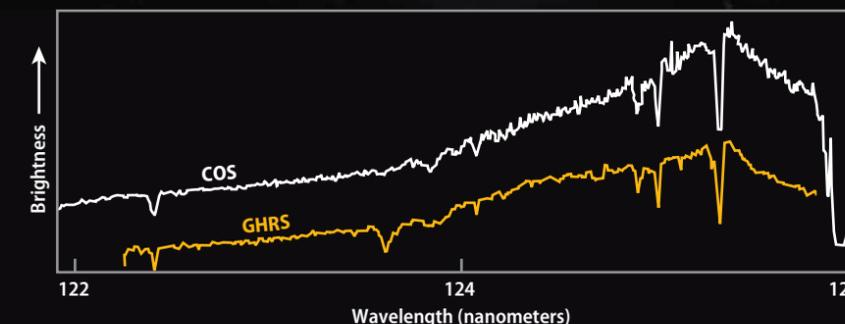
**Active galaxy Markarian 817** shows off the expanded capabilities of the new COS instrument. This view compares a COS spectrum with that from one of its predecessors, the Goddard High Resolution Spectrograph (GHRS). COS is 10 times more sensitive than GHRS, so it records more light and has a higher signal-to-noise ratio. This view also shows all the wavelengths captured by GHRS but only one-eighth of those COS records. WFC3 photographed the galaxy (top).
