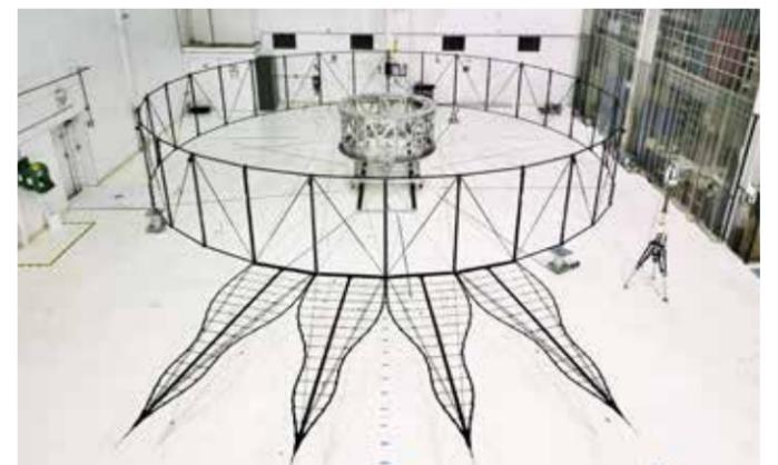
▲ Researchers are working on a prototype starshade. This 34-meter-wide instrument would block the light from a distant sun, allowing the orbiting planet's reflected light — about 10 billionth the brightness — to be visible. JPL
