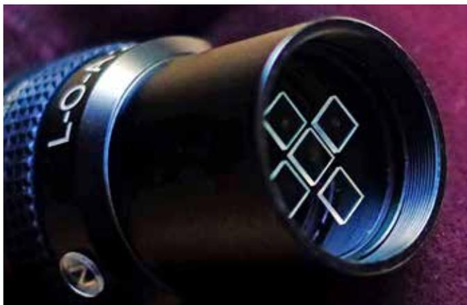
This glass array, which Denkmeier attached to one of the eyepiece's field lenses, creates the 3-D effect.
