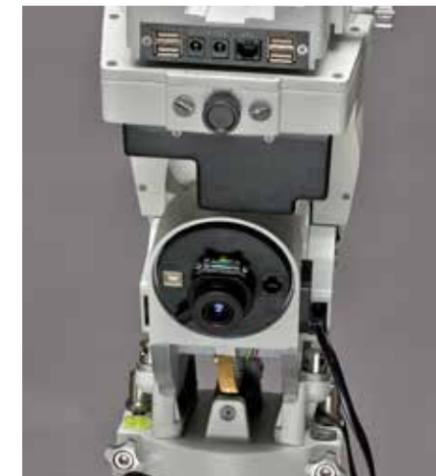
When the view through the included polar alignment scope matches the one "Quick Polar Alignment" shows you, the drive is aligned to our planet's rotational axis.
