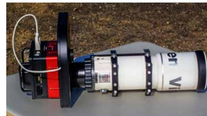
Using a custom adapter, the author connected his SBIG STX-16803 CCD camera to Vixen's VSD100F3.8 optical tube assembly with no problems. TONY HALLAS
