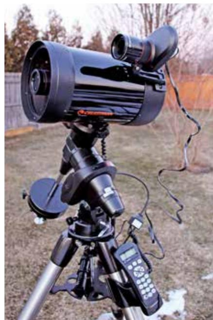
The author attached the StarSense to his Celestron C6 telescope. This instrument rides on an older CG-5 mount, which required Celestron's AUX Port Splitter. PHIL HARRINGTON
