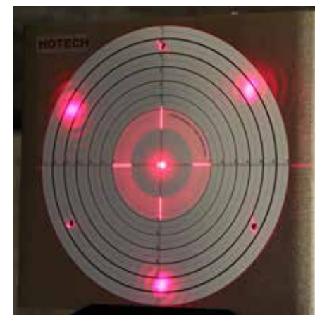
The light from the lasers enters the telescope and returns to the target. At this point, you'll know if the scope's alignment needs tweaking. TOM TRUSOCK
