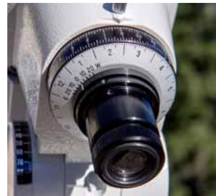
The GPD2 mount features an internally illuminated polar-alignment scope. TONY HALLAS
