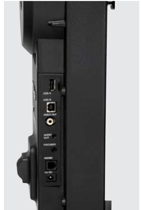
The accessory panel of the ETX-LS offers audio and video outputs, a focuser control, and two USB ports.
