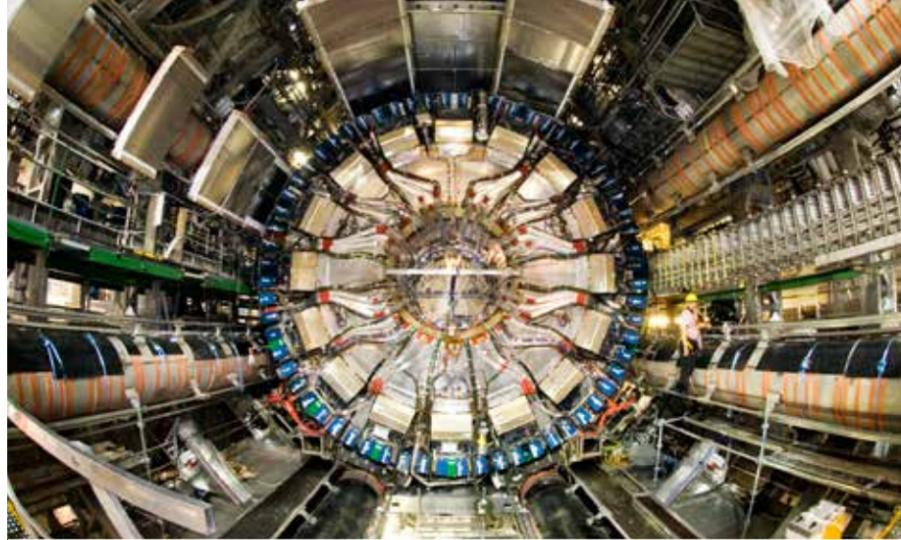
**SCIENTISTS AT CERN** will use the Large Hadron Collider's ATLAS detector to smash together high-velocity proton beams. The resulting subatomic debris should reveal fundamental particle processes. The ATLAS experiment is one of the largest collaborative efforts ever attempted in the physical sciences. The project involves 2,500 physicists from 169 institutions in 37 countries. CERN/CLAUDIA MARCELLONI
