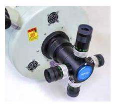
like any visual back and accepts up to four  $1\frac{1}{4}$ " eyepieces. To view through one of them, simply rotate the holder until the chosen eyepiece click-stops into position.
