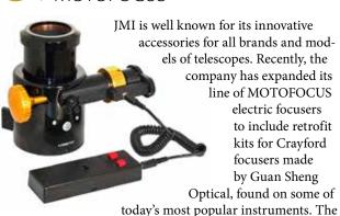
MOTOFOCUS attaches directly to the focuser without drilling. Once it's in place, just attach the hand controller to the MOTOFOCUS using the supplied coiled cable. A 9-volt battery in the controller powers the MOTOFOCUS' motor, while push-buttons on the box control the direction of focuser travel. A three-position switch adjusts the focusing speed.
