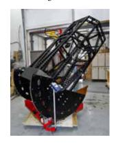
the elliptical secondary, lowers the height of the eyepiece by about 50 percent, which means most observers can reach the eyepiece by climbing only three steps. The open truss instrument comes equipped with the ServoCat/Argo Navis GoTo System. And despite the telescope weighing an estimated 1,400 pounds (635kg), a person can move it in altitude or azimuth with just one finger.
