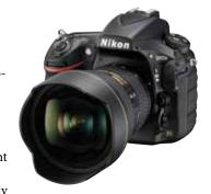
constructed optical filter it attaches to the front surface of the camera's 36-megapixel CMOS sensor to gain four times greater transmission of H $\alpha$  than its standard D810. The D810A, like its predecessor, can enlarge the live view through the lens up to approximately 23x for better focusing accuracy.
